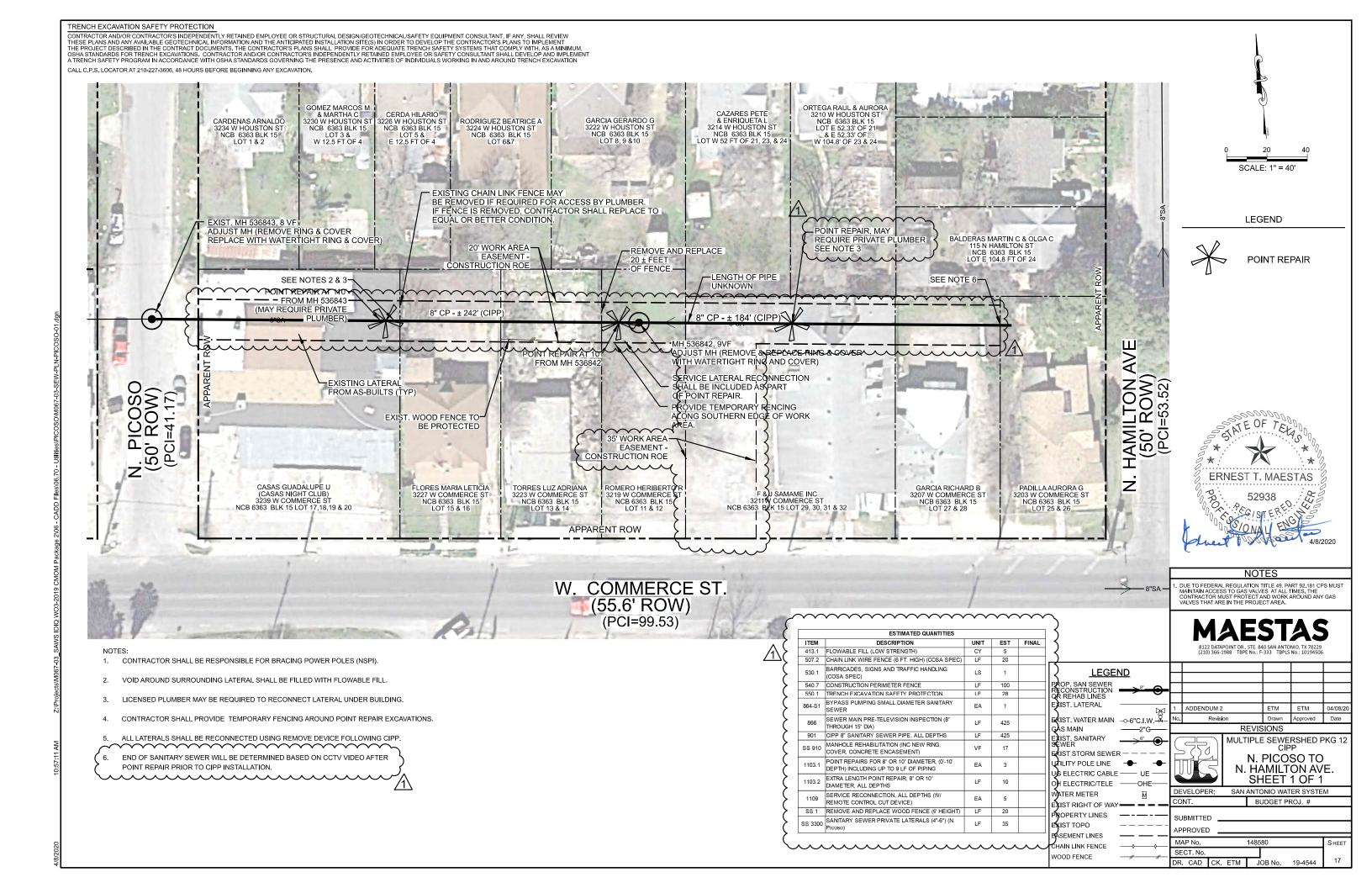
CONTRACTOR TO COORDINATE WITH PROPERTY OWNERS TO MINIMIZE SEWER FACILITY USAGE DURING CONSTRUCTION AND/OR INTERCEPT SEWER LATERALS AS NEEDED.
