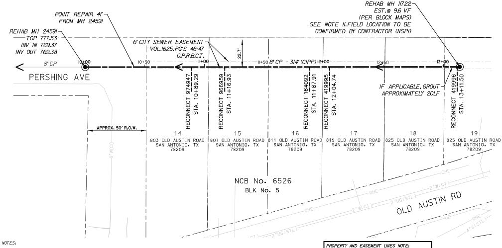
PROPERTY LINES AND EASEMENT LINES ARE SHOWN AT APPROXIMATE LOCATIONS BASED ON GIS DATA (APPARENT ROW) AND SHOULD BE
